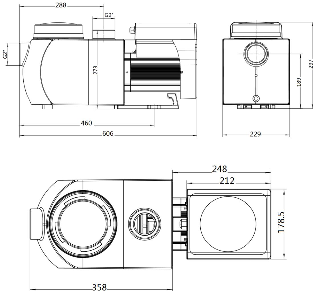
Figure 1: Overall product dimensions in mm
